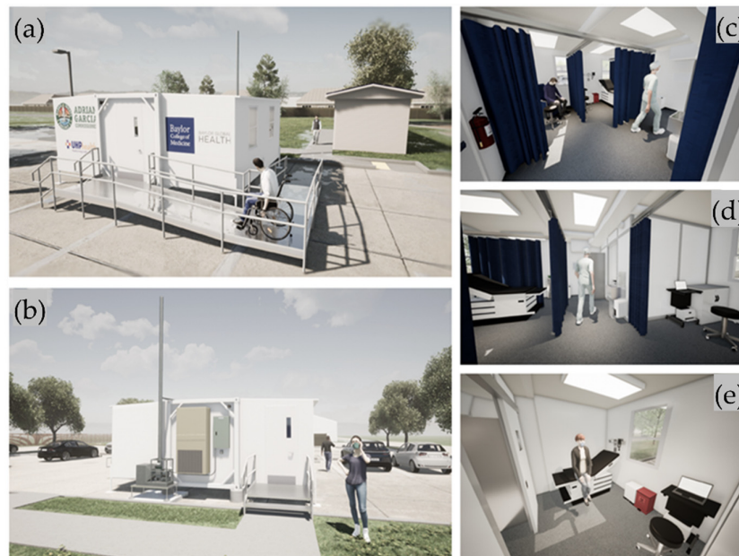
Figure 1. Illustration of a 3D-rendered model of the COVID-19 Smart Pod isolation clinic. (a,b) Exterior of the portable, expandable container unit: entrance and exit, respectively; (c,d) Interior: patient examination area (Exam Rooms 2 and 3) separated by disposable antimicrobial curtains and check-in area (positive pressure zone); (e) Negative pressure isolation room (Exam Room 1).
